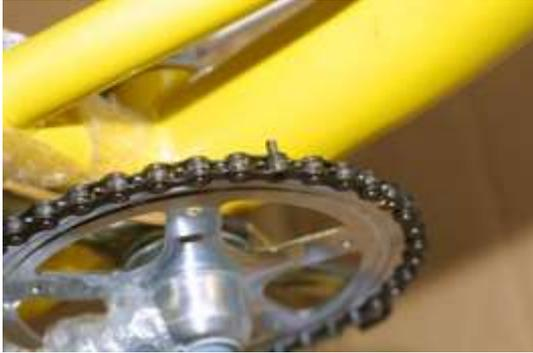
The chain is threaded through the rear gear cluster, through the chain tensioner and then back up to the front sprocket. Each end of the chain is held together by a metal pin which is pushed through the chain link to secure the chain correctly.
