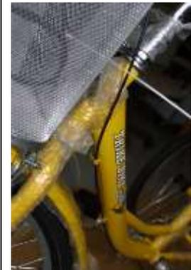
The gear change cable goes from the right-hand handlebar over the top of the basket support and then fits into the cable guides as shown in the photograph. There are several of these which support the cable down underneath the frame and past the pedals to the rear of the frame.
