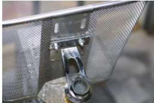
The front basket attaches to the top of the steering yoke as shown in the photographs
