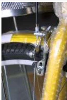
Connecting the front brake cable is very easy. Make sure the cable is properly seated on the right handlebar and run it down to the front brake as shown in the photograph.
