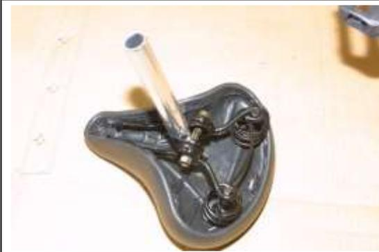
Locate the Trike-Bike™ seat and also the seat support pole and fit as shown in the photograph, tighten the 13mm nuts on both sides so the seat so it's clamped firmly onto the seat support pole.
