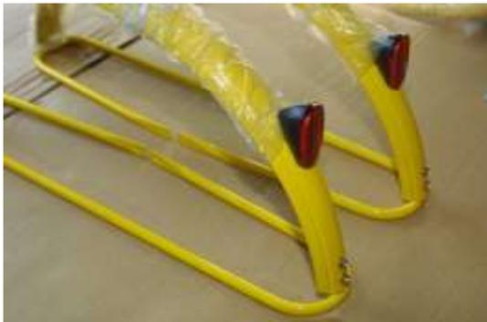
Fit the rear mud guards to their support brackets as shown in the photograph. At this stage do not tighten the bolts which secure the rear mud guards to the frames.
