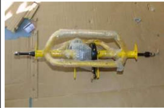
Locate and partially unwrap the main rear axle assembly. Remove the bubble wrap from the end of the axles as shown in the photograph.
