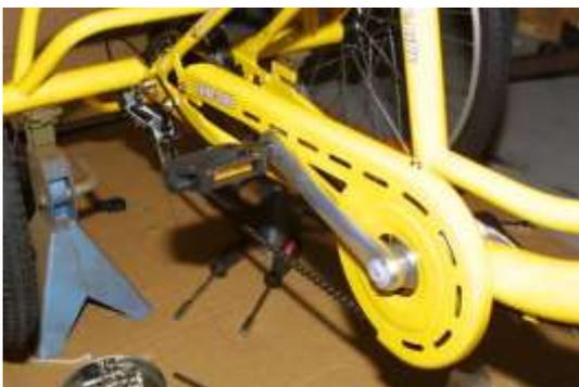
Fit the chain guard (3 bolts) and then fit the right hand side pedal into position.
