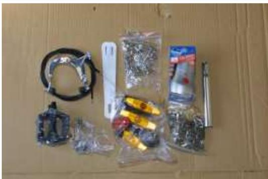
In the small box shown in the bottom left-hand corner of the photograph above is all of the hardware required to assemble the bike including LED light, chain, seatpost, reflectors, front brake, brake cables, pedals and other associated hardware, nuts and bolts etc. for the assembly.
