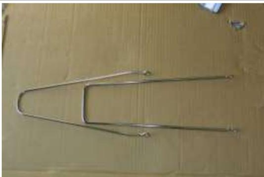
Locate the two chrome support frames which go on the front mud guard and also on the front basket.
