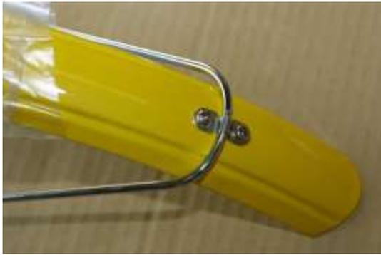
Locate the necessary hardware to fit the front support bracket to the bottom rear of the front mud guard as shown in the photograph. Make sure everything is aligned correctly and centrally before tightening the nuts and bolts.
