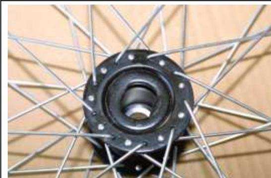
Please locate both of the rear wheels. They are similar in every respect except one wheel has a special cut out as shown in this photograph on the inside of one of the hubs. This cut out meets with a special hub which is only on one side of the main axle assembly. This alignment determines which wheel is the left wheel and which wheel is the right wheel.
