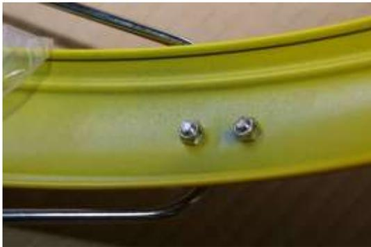
This is a rear view of the front mud guard showing that nylock nuts are used to secure this bracket in place.
