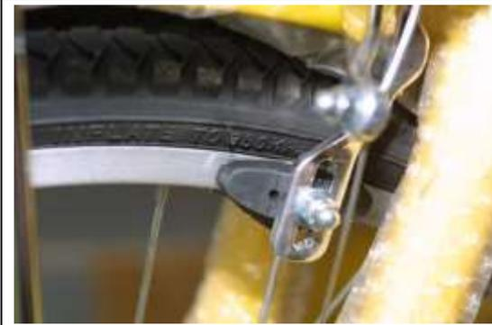
The front brake rubbers which rub against the wheel rim to provide you with stopping power need to be adjusted into the correct position as shown in this photograph.
