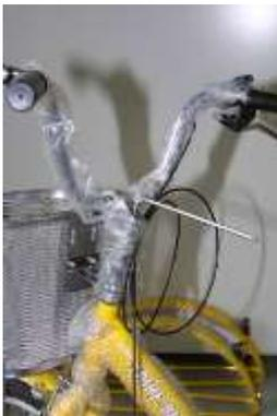
The front handlebar assembly is now fitted into the front fork assembly, everything is aligned so it is right angles to the front wheel and then the handlebar unit is secured by tightening the hidden bolt with the allen key as shown in this photograph.
